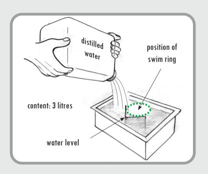
Fill up the water container with distilled water until you reach the top edge of the inner metal bracket.
