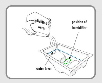
Fill up the water container with distilled water until you reach the water level.
